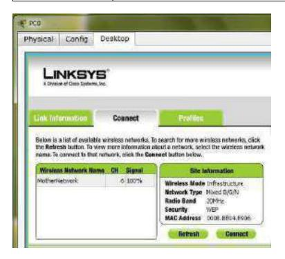
As you can see in image that Wireless device is accessing MotherNetwork on CH 6 and signal strength is 100%. In left side you can see that WEP security is configured in network. Click on connect button to connect MotherNetwork
